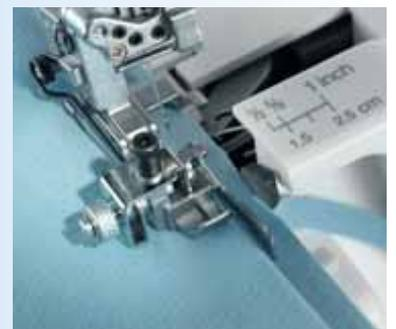
**4 |** Make sure the needle barely pierces the fabric fold on the left. The needle should only pierce one or two fibers of the fabric while sewing! The further left the needle pierces the fabric, the more visible stitches become on the right fabric side.
