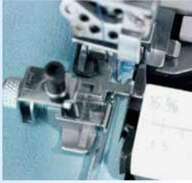
**5 |** The blind hem foot can easily be adjusted for sewing perfect, invisible hems on different types of fabric: **After having found the optimal positioning of the hem, turn the adjustment screw on the presser foot forwards or backwards to move the foot's guide plate until it lines up with the edge of the fold.**
